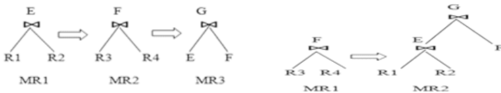
Figure 5: Represent of the Query Plan 1 and Query Plan 2 (as shown in figure 3) In MapReduce (Chen, Y., et al., (2014)
